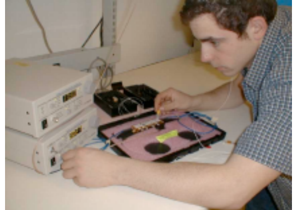
Students use purchased and donated components to fabricate and test a WDM system at two wavelengths.
