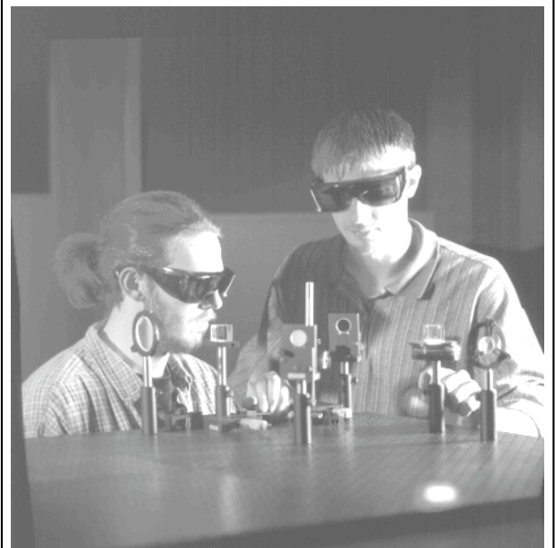
Jason Patch and Shawn Percy make adjustments to a Mach-Zehnder interferometer as part of the Advanced Laser Topics course.
